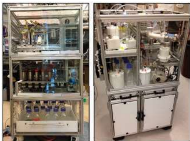
▲ Figure 7. This modular plant can manufacture a variety of pharmaceutical products on-demand (4).
